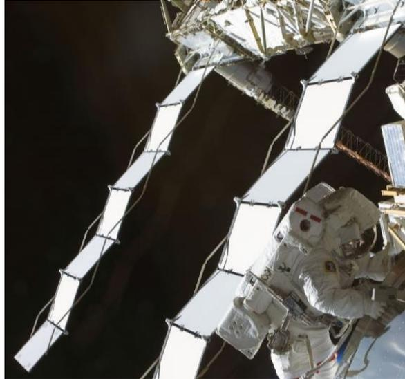
Figure 5: Radiators that are used to emit heat from the ISS into space [7]
