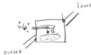
Figure C9: Heating the sample via induction, coiled heater above sample.
