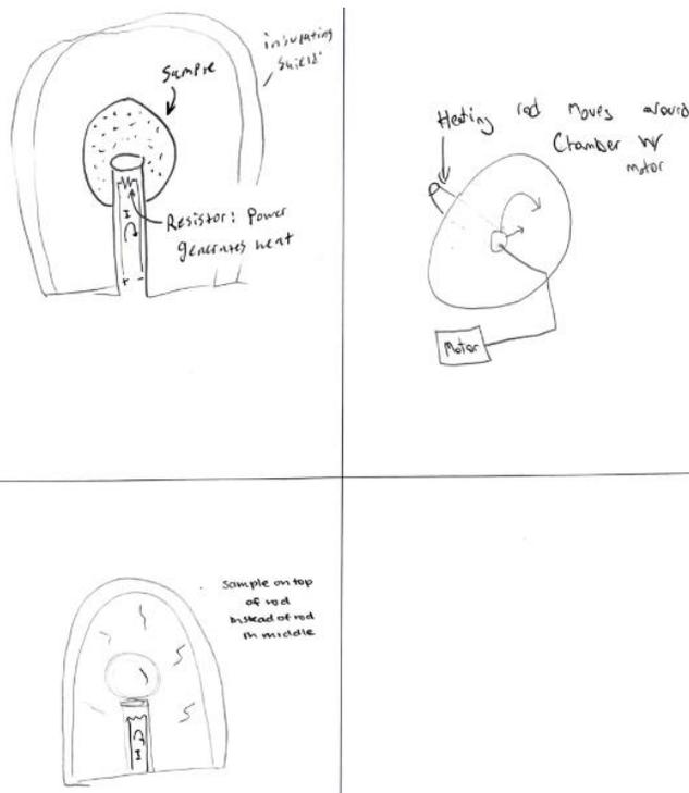
Figure C3: This system uses conduction through one rod, constantly “stirring” the sample.
