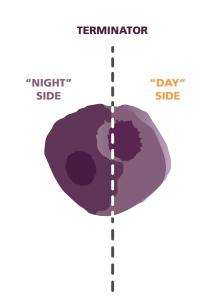
We only want to take images while the spacecraft is in the light, so these "terminator crossing" geometric events are what we use to determine the timing of the imaging observations. We must take advantage of every moment that the spacecraft is on the day side of the asteroid. Timing is crucial. But because we are still uncertain about the exact timing, we actually need to plan to start taking images a little before the spacecraft crosses from dark to light.
