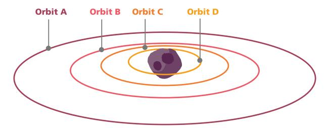
In **Orbit A**, the spacecraft will take 32.5 hours to complete a single circuit. For half of that orbit, the spacecraft will be on Psyche's day side, observing the surface of the asteroid for about 16 hours. Then, when it's on the night side, the spacecraft will point its main antenna toward Earth and send back all of the data it just acquired. Thus, every 16 hours or so, we will receive the data that the spacecraft collected while it was on the asteroid's day side.
