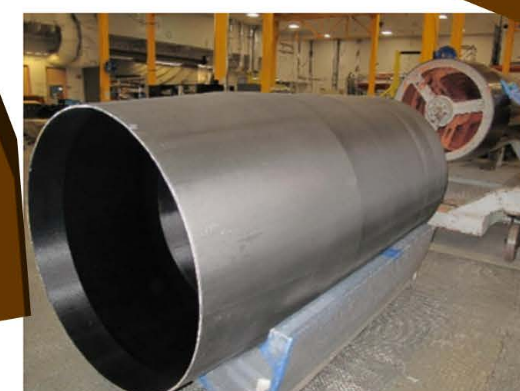
Figure 13: Central Cylinder Structure for the Psyche Spacecraft
